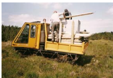
Figure 17. Using a Muskeg to transport material to the monitoring point at Bellaveeny.
