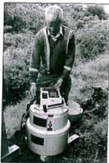
Water quality is being monitored downstream of the site using an autosampler
